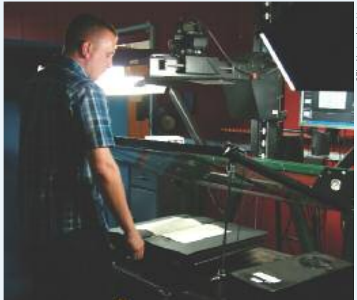
Camera station with integral book cradle and adjustable glass plate
